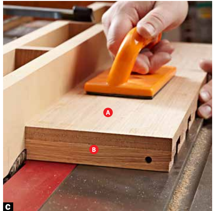
C A rabbet along the ends of the spacers mimics the gap above and below the hooks so they all blend together.
